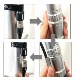
Before replacing the handpiece, make sure the device is turned off. Connect the white part of the handpiece cable to the arm cable and insert. Connect the handpiece to the arm while rotating.
